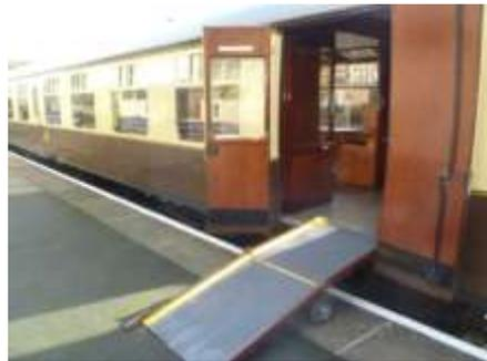
**Standard single carriage door with steps (left) and ramp access to double doors**
